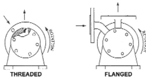
**Figure 1:** Direction and Port Location
