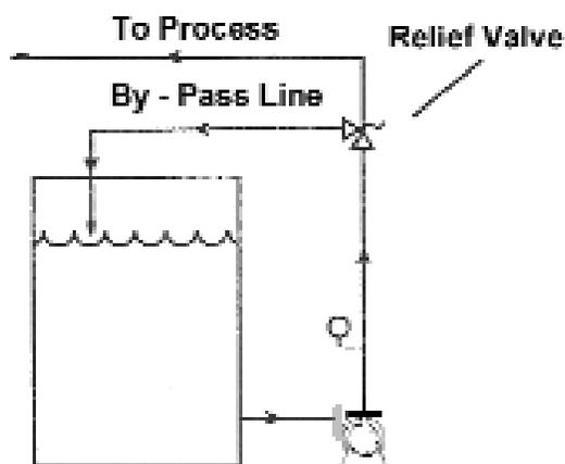
**Figure 2:** By-pass Configuration
