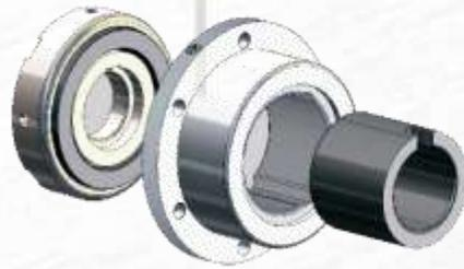
Field assembling of the product lubricated bearing assembly does not require special tools. The bearing material is available in Silicon Carbide (SIC), or Tungsten Carbide (TC), to meet specific conditions. The use of tolerance rings reduces the sleeve bearing and thrust bearing loads to withstand system upsets without failure, and ensure many years of maintenance-free operation.
