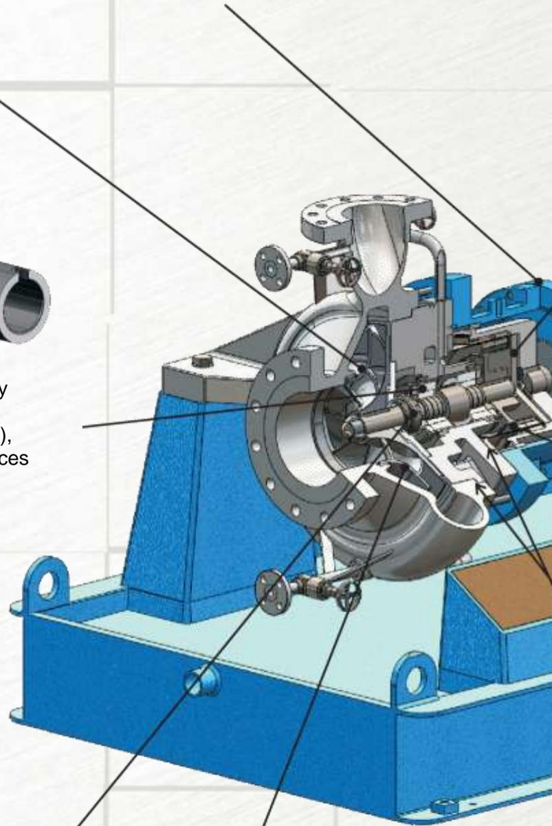
REAR CARTRIDGE KIT with registered fits for quick and easy maintenance procedures.
