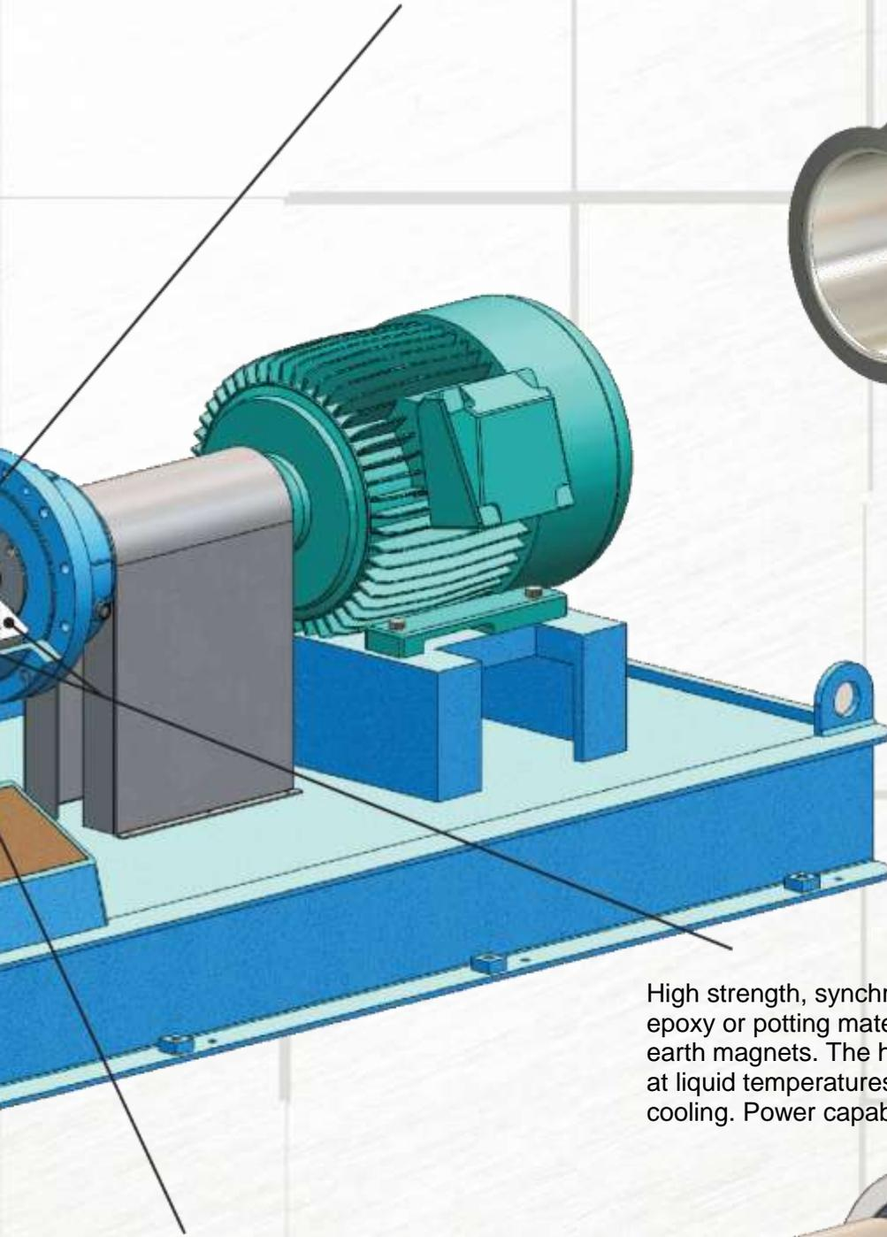
High strength, synchronous magnetic couplings, are free of epoxy or potting materials, and fitted with samarium cobalt rare earth magnets. The high performance magnets can be operated at liquid temperatures up to 662 °F (350 °C) without external cooling. Power capability exceeds 700 HP / 520 kW.
