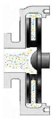
Disc-rotor pumps employ pumping action, with a minimal contact between the fluid and internal pump surfaces.
