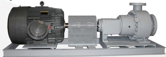
The appearance is similar to centrifugal pumps, minus the internal friction and wear associated with conventional impeller vane technology. VSS discrotor pumps function like centrifugals, and are more versatile than progressive cavity (PC), rotary lobe and gear configurations. VSS pumps deliver flows from 2 to 6,000 GPM and heads to over 4,000 ft.
